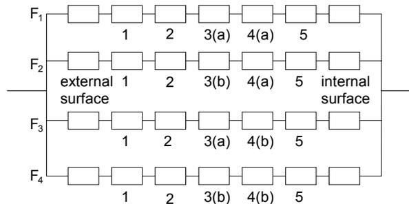
Resistance through section containing AAC blocks and mineral wool
