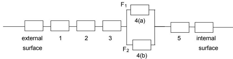
The lower limit of resistance is then obtained by adding up the resistances of all the layers:
