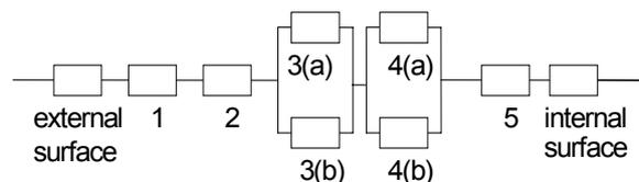
The resistances of the layers are added together to give the lower limit of resistance. The resistance of the bridged layer consisting of AAC blocks and mortar is calculated using:
